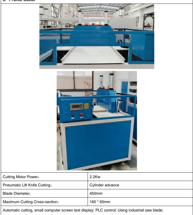
Adopts fine tooth saw blade, which cutting surface formation. Cutting speed will be adjust by the throttle, and
